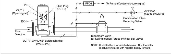
NOTES: 1. With a spring-loaded torque cylinder ball valve, the tubing runs same as that with a diaphragm valve. 2. In combining with a diaphragm valve or spring-loaded torque cylinder ball valve, stop up OUT 2 with a blind plug.
